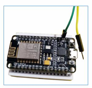
Now connect the yellow wire of the LED to the Node MCU D1 pin as shown in the image given below.
